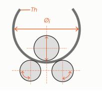
Rolling shall be performed in following conditions :  $\emptyset I \ge 40$  th (temperature of the piece  $\ge 10^{\circ}C - 50^{\circ}F$ )
