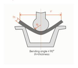
Ri : Min internal bending radius
